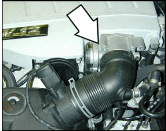
J338 Throttle Valve Control Module (6.0 liter engine)
