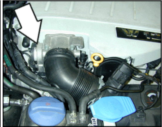
G297 Angle sensor 1 (on throttle drive 2 power accelerator actuation) (6.0 liter engine)
