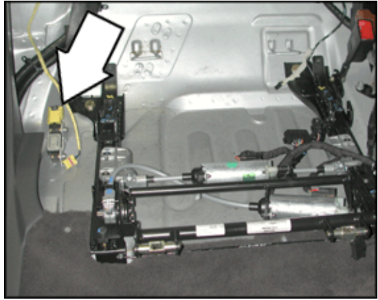
G257 Right Rear Side Airbag Crash Sensor
