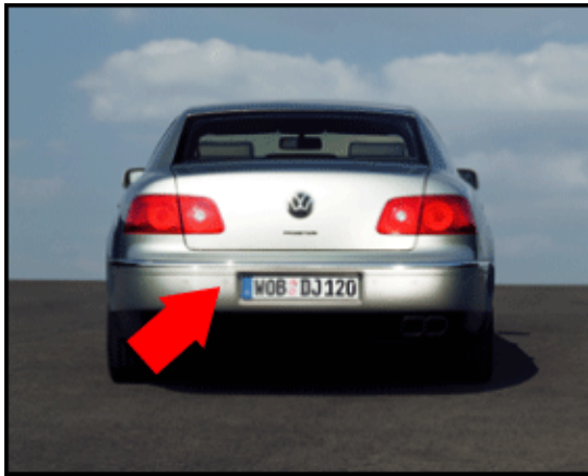
G334 Left Rear Inner Parking Aid Sensor
