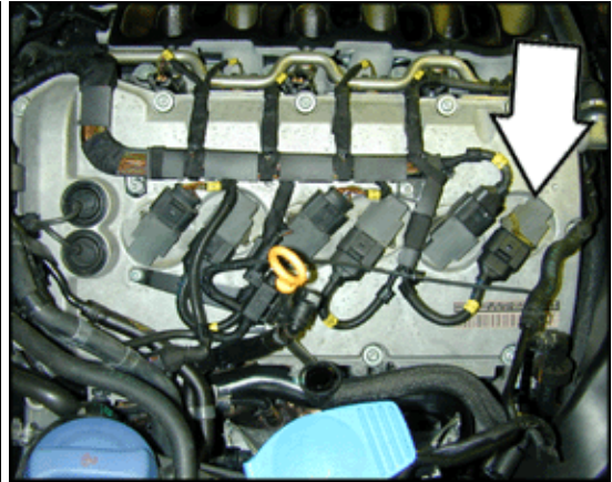
N70 Ignition Coil 1 with Power Output Stage (6.0 liter engine)
