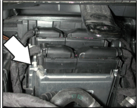
J624 Engine Control Module 2 (6.0 liter engine)
