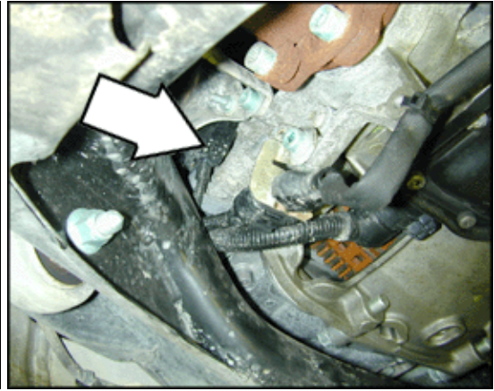
G28 Engine Speed (RPM) Sensor (6.0 liter engine)
