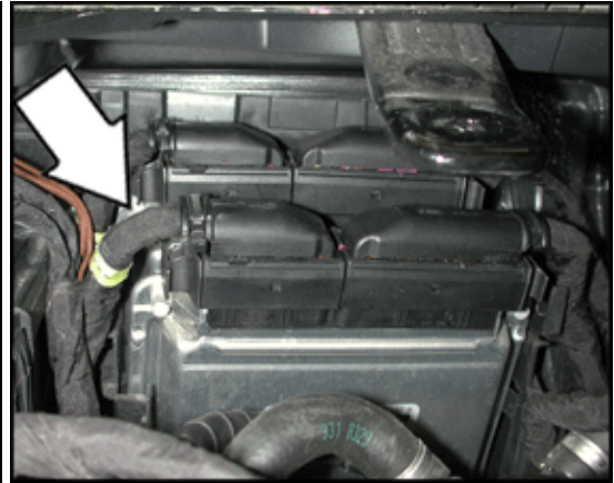
J623 Engine Control Module (ECM) (6.0 liter engine)
