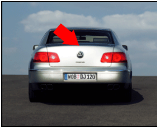
R137 Luggage Compartment Access/Start Authorization Antenna
