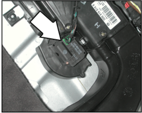
V195 Right Rear Footwell/Defrost Flap Motor
