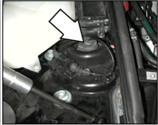
N337 Right Front Dampening Adjustment Valve
