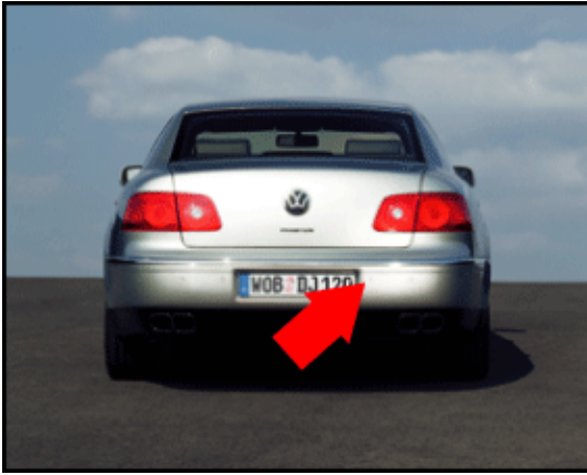
G335 Right Rear Inner Parking Aid Sensor
