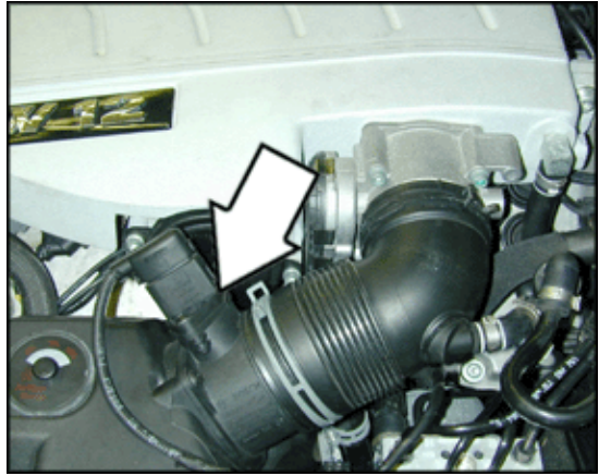
G42 Intake Air Temperature (IAT) Sensor (6.0 liter engine)
