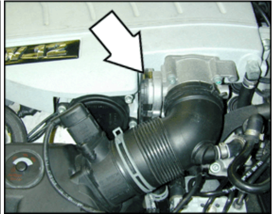
G187 Angle sensor 1 for throttle drive (power accelerator actuation) (6.0 liter engine)
