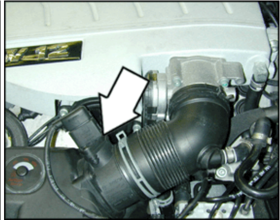
G70 Mass Air Flow (MAF) Sensor (6.0 liter engine)
