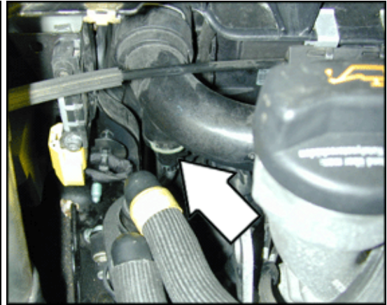
G83 Engine Coolant Temperature (ECT) Sensor (on Radiator) (6.0 liter engine)
