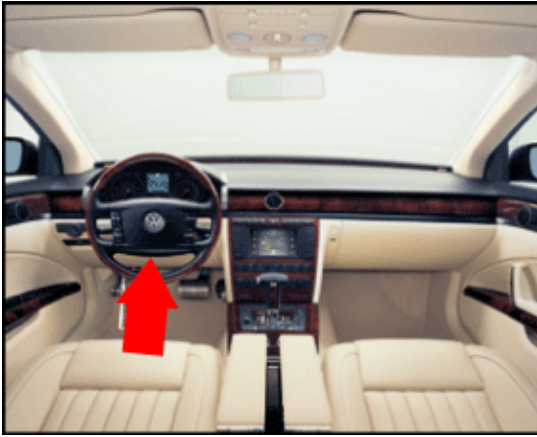
G357 Steering Column Vertical Adjustment Sensor
