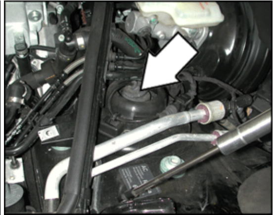
N336 Left Front Dampening Adjustment Valve
