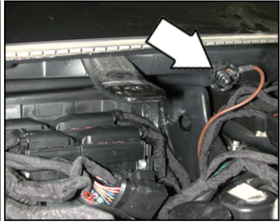
647 Ground Connection 3 (on bulkhead)
