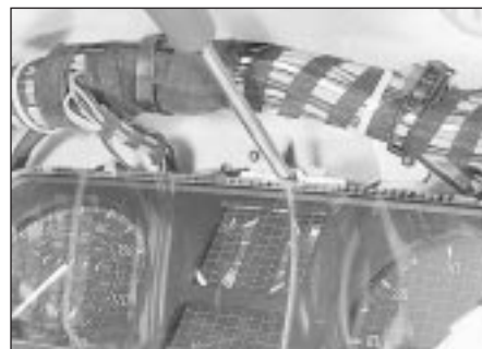
8.7a Removing the instrument panel securing screw
