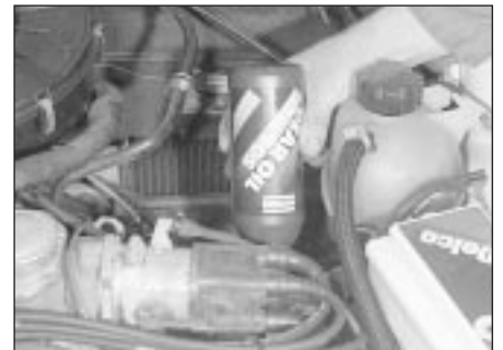
27.4b . . . then top up via the breather/filler plug orifice
