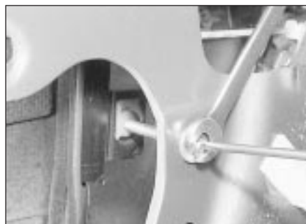
19.6 Adjusting the rear window guide rail There is another locknut behind the panel
