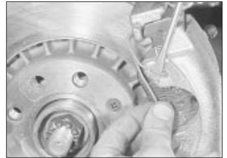
4.17 . . . then lever out the spring clip
