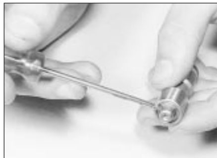
10.13b Locate the cap flange in the plunger groove
