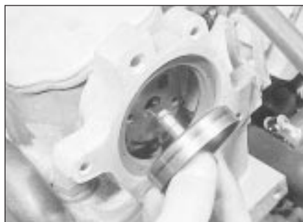
3.11a Extract the rotor hub . . .
