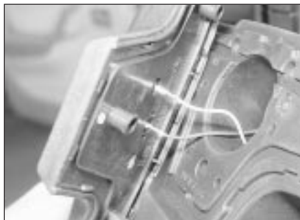
19.2 Removing the steering wheel central cap
