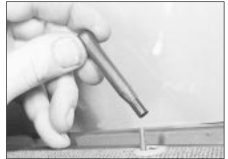
12.4 Unscrewing the lock button
