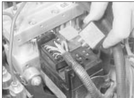
22.16a Removing the relays from the hydraulic unit
