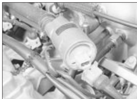
12.44a Disconnect the idle speed adjuster multi-plug . . .
