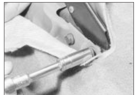
19.5 Unbolting the handbrake lever
