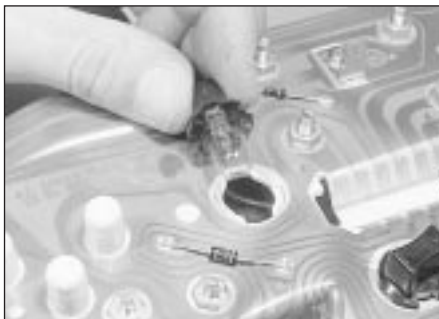
11.27 Removing an instrument panel bulb
