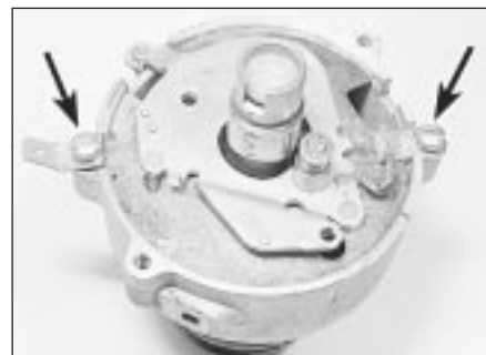
7.7 Undo the baseplate retaining screws (arrowed)
