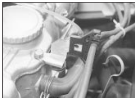
8.29b HT lead bracket is secured by one of the camshaft cover bolts
