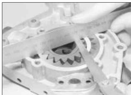
14.3 Checking oil pump gear endfloat
