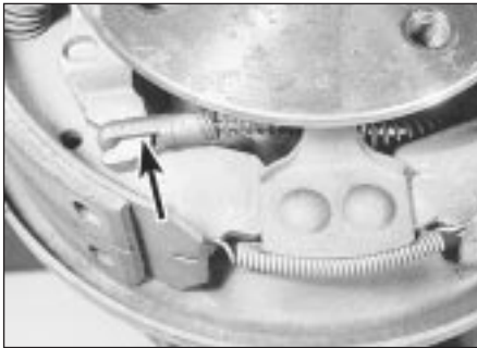
6.6 Handbrake cable attachment to operating lever (arrowed)
