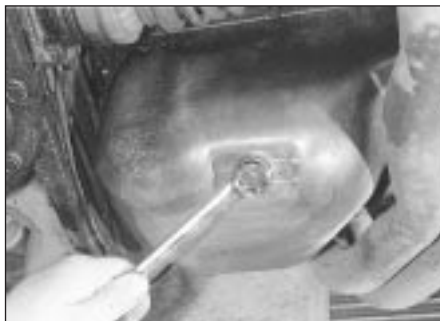
6.4 Removing the sump drain plug
