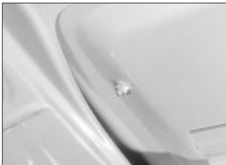
26.9 Boot lid handle retaining nut
