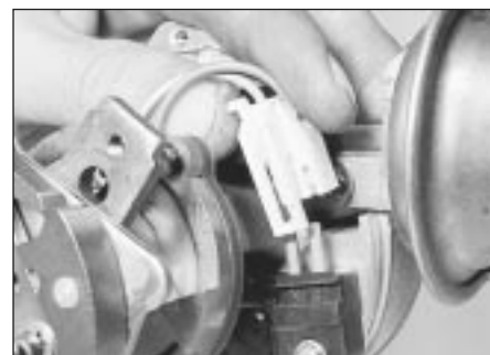
4.3 Disconnecting an electrical plug from the ignition module
