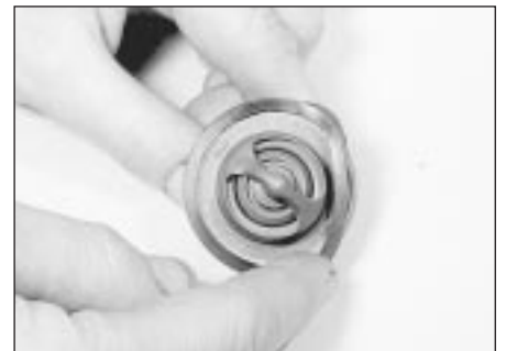
4.14 Fitting a new seal to the thermostat
