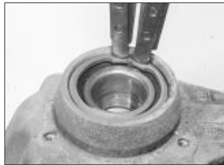
3.5b Removing a hub bearing circlip
