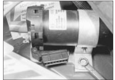
6.4a Removing a coil securing bolt
