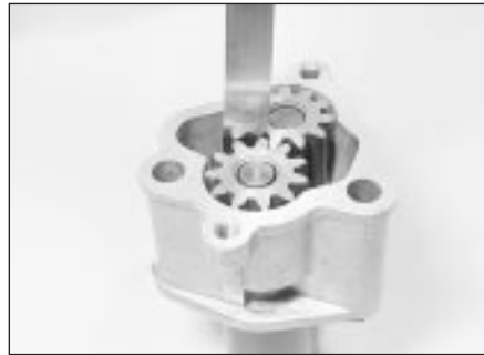
13.8 Check the pump gear teeth backlash
