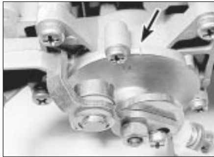
14.5 Notches on choke cover and carburettor housing (arrowed) aligned
