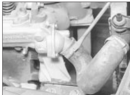
4.8 Slackening the hose clip at the thermostat housing (1.6 litre model shown)
