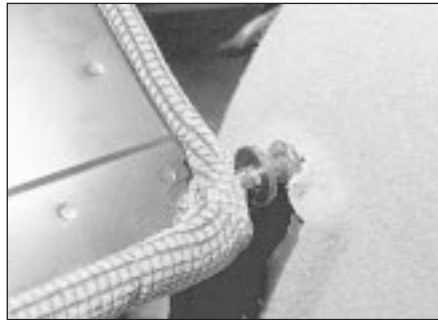
33.3b Seat pivot lifts out of hinge
