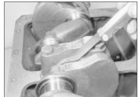
20.18 Checking the crankshaft endfloat
