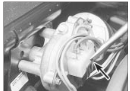
20.6 Releasing the wiper motor electrical plug
