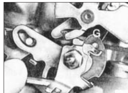
16.21 Full throttle opening adjustment - bend tang G to adjust choke gap
