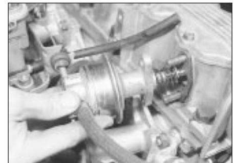
5.5 Removing the fuel pump (1.3 litre engine shown)
