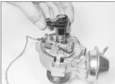
4.2 Removing the rotor arm
