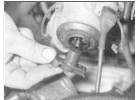
10.9b . . . and pull off the rotor arm from the distributor shaft (1.6 litre model shown)
