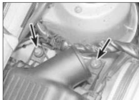
2.5a Two of the air cleaner securing bolts (arrowed) - 2.0 litre 16-valve
