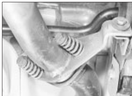
14.5 Manifold-to-exhaust system joint and bracket
