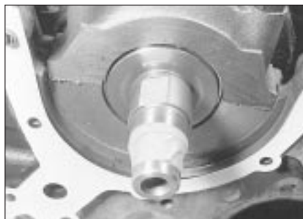
13.6 Tape the crankshaft nose
