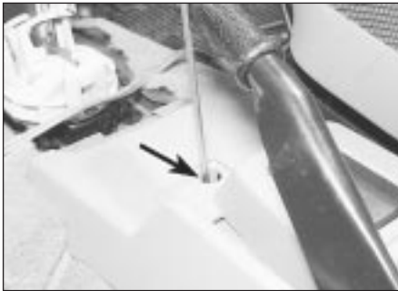
35.2b Removing the centre console rear half screw
