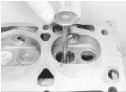
9.15 Fitting a valve to its guide
