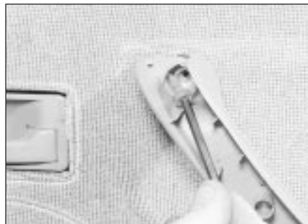
12.6b Removing an armrest screw
