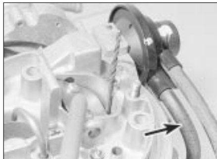
15.9a Checking the choke pull-down gap. Apply vacuum to hose arrowed
