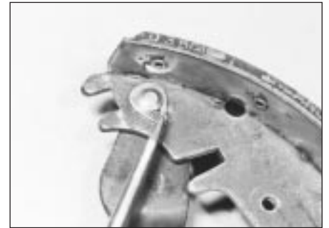
6.16 Handbrake lever secured by pin
