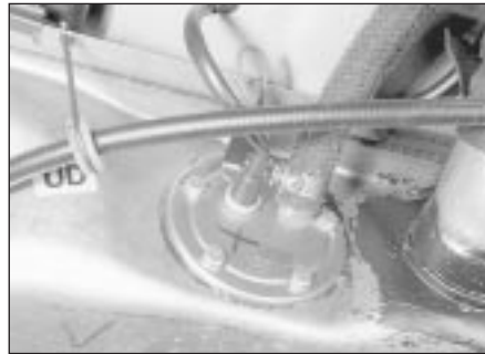
6.3 Fuel gauge sender unit secured by bolts
