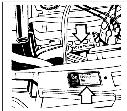
Engine number and VIN plate locations (arrowed)
