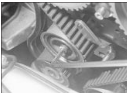
7.10 Slackening the camshaft belt tensioner screw
