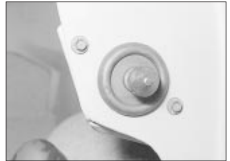
33.5a Seat backrest catch striker - Hatchback
