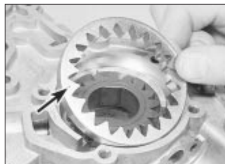
14.4 Gear outer face identification mark (arrowed)
