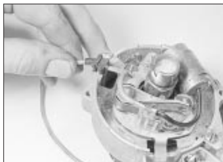
7.3 Removing the LT lead
