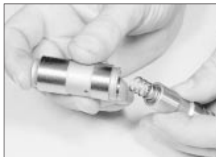
10.14b . . . then slide the plunger and spring assembly into the cylinder
