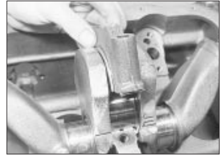
20.14 Fitting the centre main bearing cap
