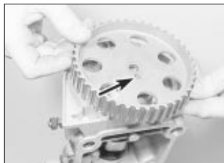
9.12a Fitting the camshaft sprocket. Peg locating hole is arrowed
