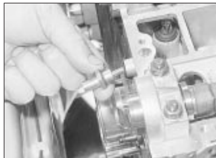
11.18b . . . and the belt cover mounting stud
