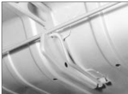
25.5a Torsion rod central housing bracket
