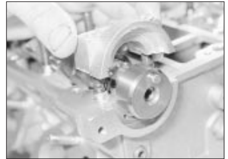
10.11 Fitting a camshaft bearing cap
