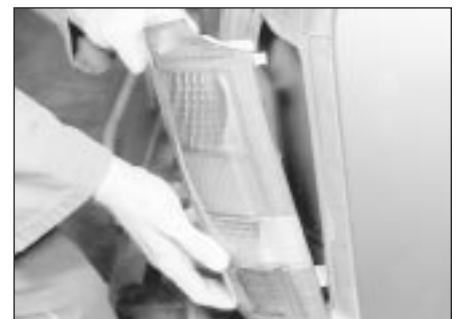
11.17b Removing a rear lamp lens
