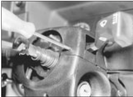
20.3a Removing an upper shroud securing screw
