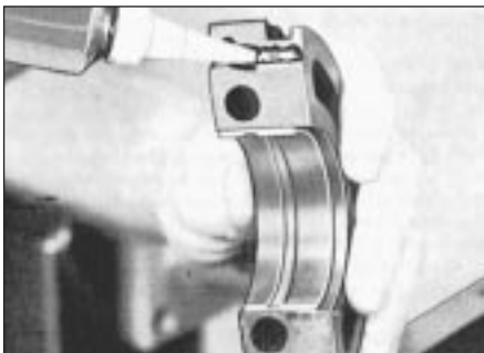
20.15b Fill the rear main bearing cap grooves with sealant
