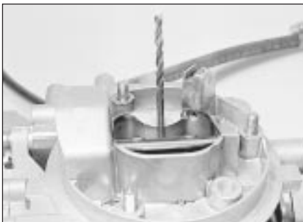
14.8b Measuring the choke valve gap using a twist drill
