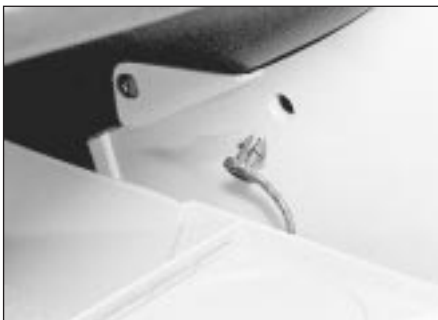
36.1 Glovebox check strap disconnected
