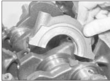
20.16a Fitting a main bearing cap
