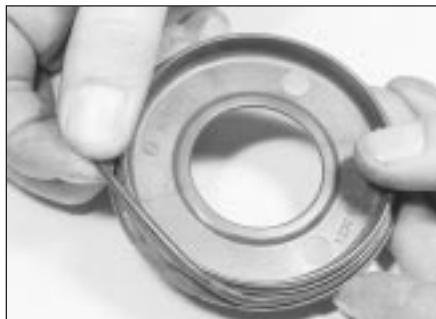
3.27 Renewing the insulator sealing ring
