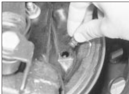
29.2 Removing the sealing grommet from the inspection hole in the rear brake backplate
