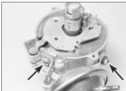
7.6a Remove the vacuum unit retaining screws (arrowed) . . .
