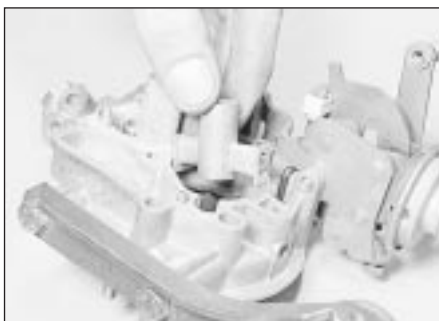
19.16 Removing the pre-atomiser
