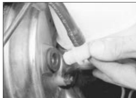
15.3 Brake servo vacuum connection at servo
