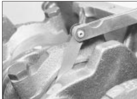
20.19 Checking crankshaft endfloat
