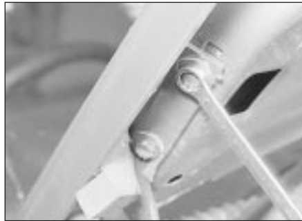
6.3 Removing a bonnet hinge bolt
