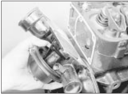
5.4 Removing the water pump - 1.2 litre model
