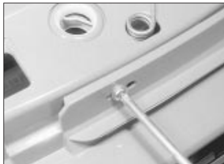
8.2 Undoing a front trim panel screw
