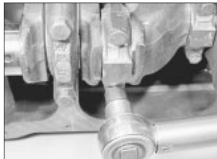
15.14b Tightening a big-end bearing cap bolt
