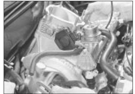
13.32 Removing the inlet manifold - 2. litre 16-valve model
