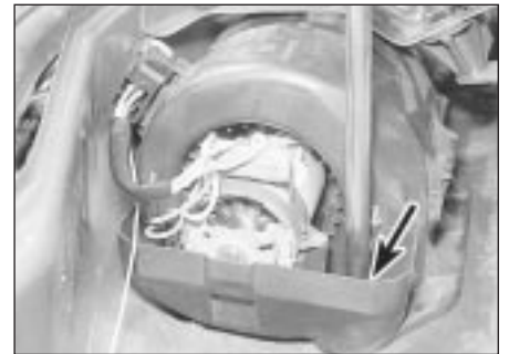
9.9 Removing a blower motor securing nut
