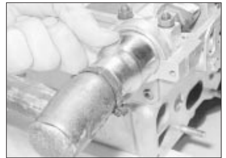
9.4b Seating a camshaft oil seal
