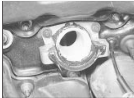
16.13a Servo mounting bracket lower half remains on bulkhead
