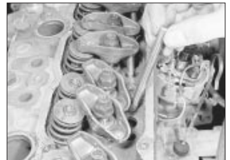
8.17 Removing the pushrods
