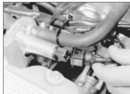
13.3d Unplugging the auxiliary air valve
