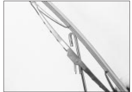
19.1 Removing a wiper blade from its arm
