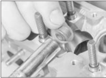
12.12a Fit a valve stem oil seal into a socket or tube . . .
