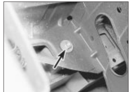
8.3 Front trim panel securing nut (arrowed)
