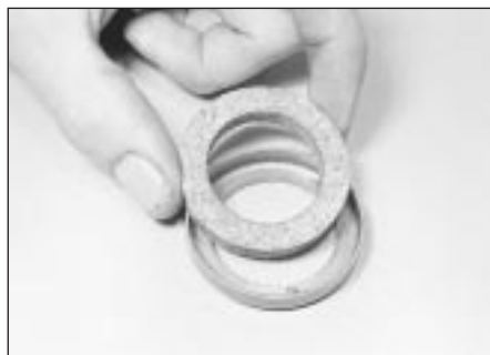
14.14a Fit the new seal to the holder
