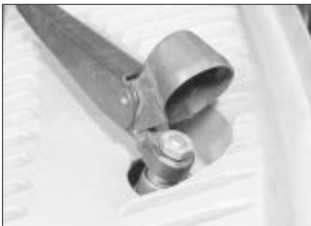
19.3 Wiper arm retaining nut
