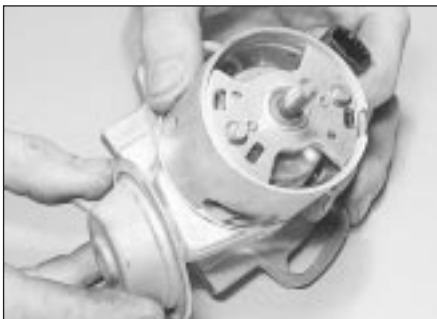
4.16b Removing the vacuum unit
