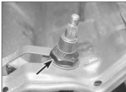
20.4 Wiper spindle clamp nut (arrowed)
