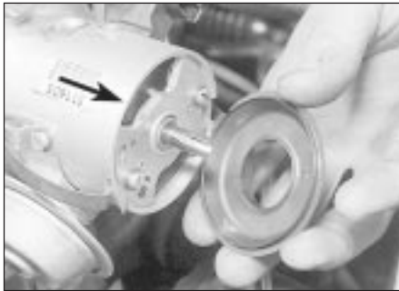
3.6c Removing the flash shield to expose the No 1 cylinder reference mark (arrowed) (1.6 litre carburettor model shown)
