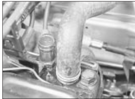
32.19a On 1.2 litre models, bleed the cooling system through the cylinder head heater hose outlet
