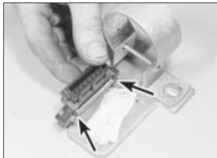
7.4 Ignition module and mounting plate - note locating pins (arrowed), and heat sink compound on baseplate (1.8 litre model)
