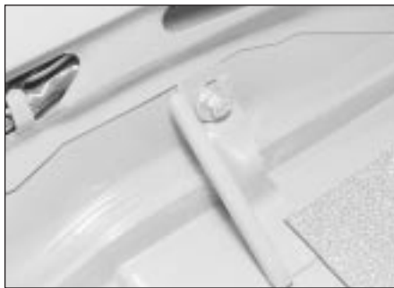
9.2 Rear trim panel securing nut
