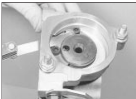
9.10 Checking the camshaft endfloat
