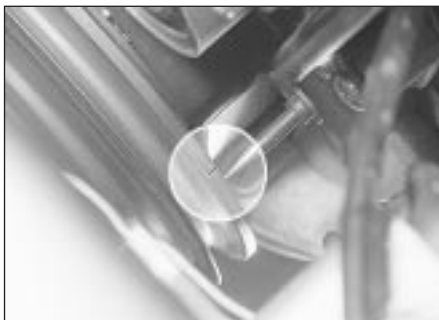
7.8a Pulley notch and pointer must be aligned . . .
