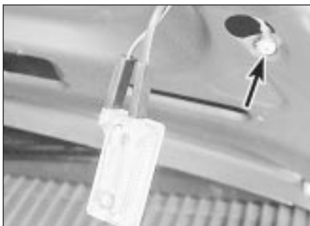
11.25a Under-bonnet lamp unclipped note earth screw (arrowed)
