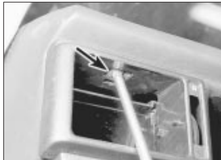
10.2 Removing a swivelling vent housing securing screw
