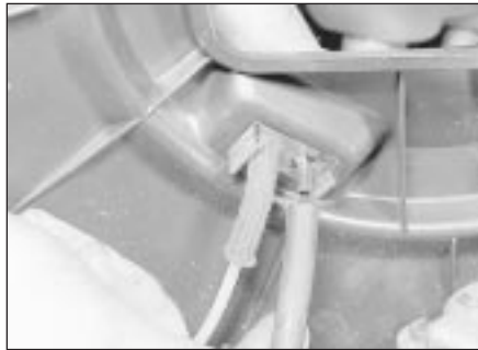
3.2b Air cleaner vacuum hose connection
