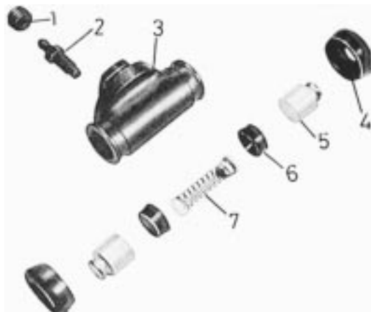
12.6 Exploded view of a rear wheel cylinder
