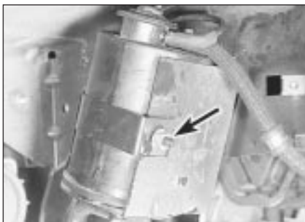
12.98a Canister clamp nut (arrowed)
