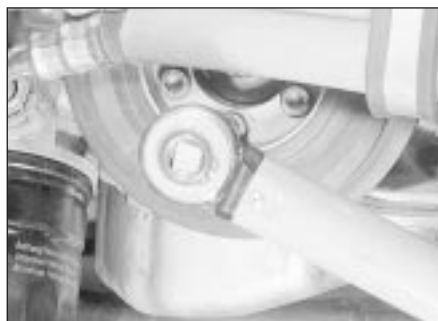
7.14 Tightening one of the crankshaft pulley screws
