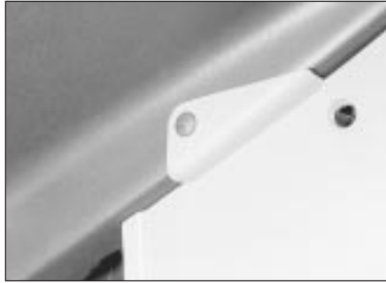
9.4b Heater control panel side screw
