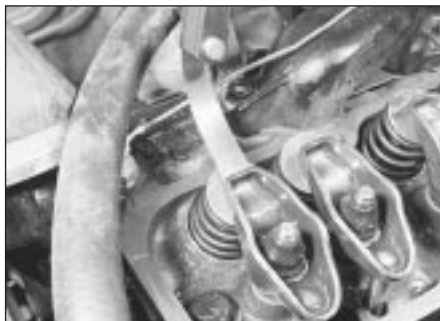
7.10 Checking a valve clearance
