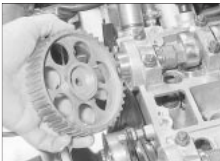
10.3b Removing a camshaft sprocket
