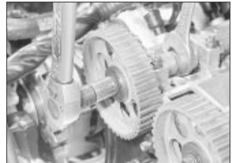
10.14 Tightening a camshaft sprocket bolt
