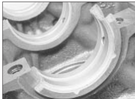
20.12 Centre main bearing shell, showing thrust flanges
