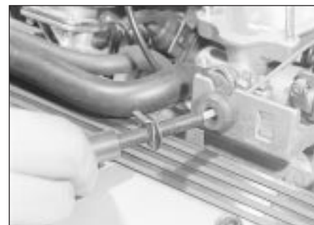
13.17 Pulling the throttle cable out of the retainer
