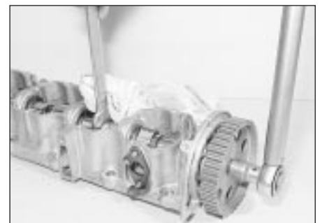
9.12b Tightening the camshaft sprocket bolt
