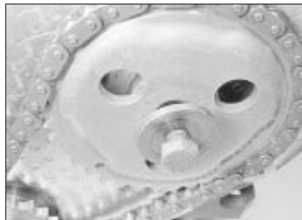
14.10 Camshaft sprocket retaining bolt and washer
