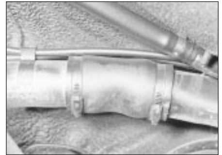
7.11 Fuel tank filler pipe-to-neck junction
