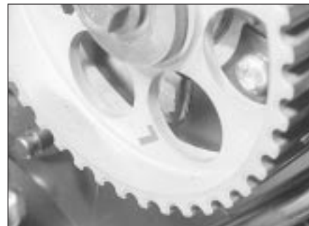
10.4 Exhaust camshaft sprocket is marked 'L'
