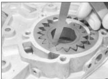
14.2 Checking oil pump gear teeth backlash
