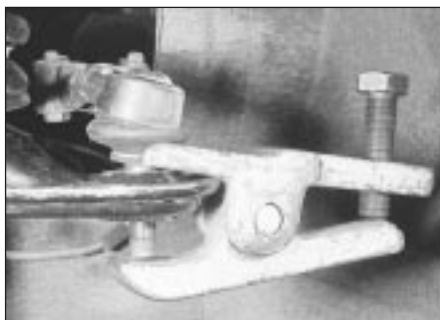
24.2 Tie-rod balljoint separator in use It is better practice to leave the balljoint nut loosely fitted
