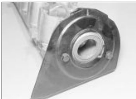
9.7 Camshaft belt cover backplate (1.3 litre engine shown)
