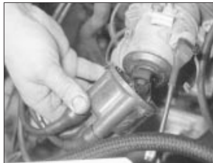
10.9a Remove the distributor cap . . .
