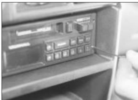
25.7 On later models it will be necessary to remove the blanking screws to be able to insert the removal tools
