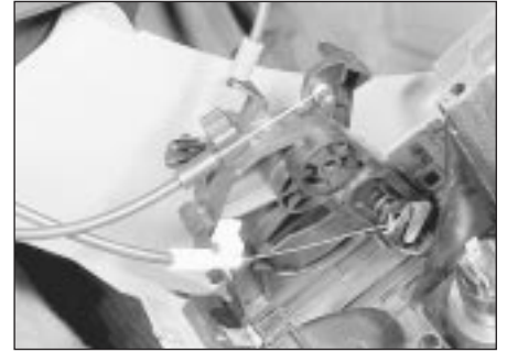
9.5 Removing the heater control panel
