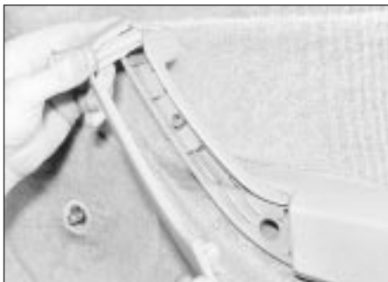
12.6a Removing the armrest screw cover
