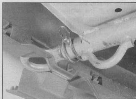
. . . then fit the shackle and secure it in position with the retaining pin
