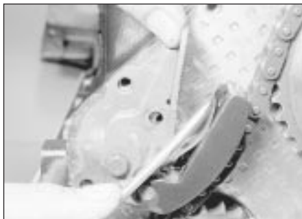
14.19b . . . then push back the spring, pivot the tensioner and fit the upper bolt
