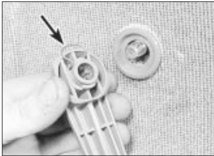
12.2 Window winder handle spring clip (arrowed)
