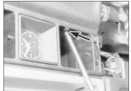
10.3 Removing a centre vent housing screw
