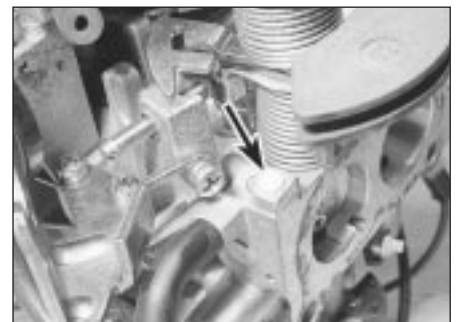
11.7b Mixture (CO) adjustment screw cap (arrowed) 2E3 carburettor
