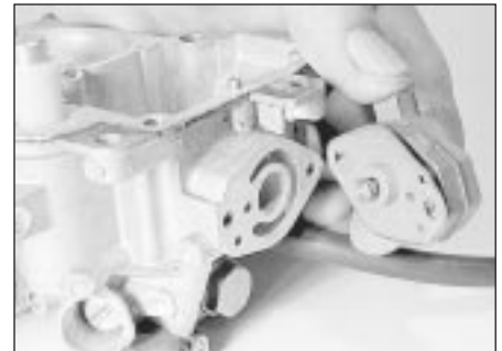
21.6 Removing the part-load enrichment device
