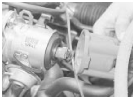
3.6b Removing the distributor cap (1.6 litre carburettor model shown)
