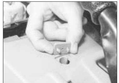
35.2a Centre console rear half screw cover
