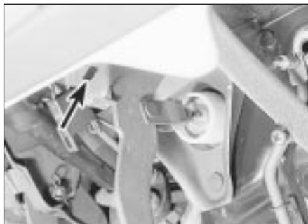
17.1 Stop-lamp switch 'keyhole' mounting (arrowed)
