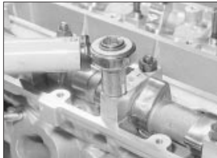
10.12 Tightening a camshaft bearing cap nut
