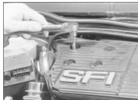
12.77 Removing a pre-volume chamber screw
