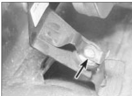
20.7 Wiper motor securing screw (arrowed)
