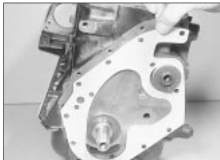
18.10 Fitting a new front plate gasket
