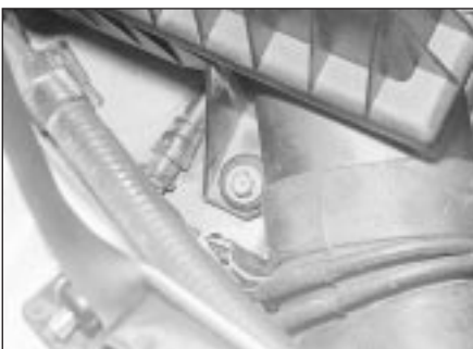
2.5b The third air cleaner bolt - 2.0 litre 16-valve
