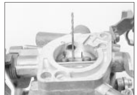
12.3 Using a drill bit to check the fast idle gap
