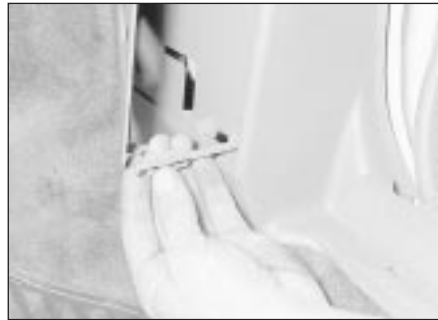
12.47 Prise out the clips to release the trim panel
