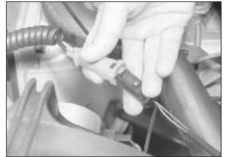
23.9b Dipstick sensor plug
