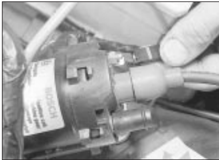
6.2 Disconnecting a coil LT lead (1.8 litre model shown)
