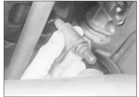
12.95 Removing the oxygen sensor
