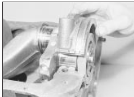
20.16 Fitting the rear main bearing cap
