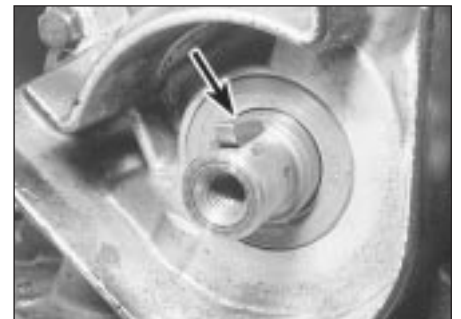
13.2b Woodruff key (arrowed) in crankshaft nose
