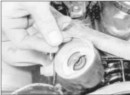
4.3a Remove the thermostat retaining snap-ring . . .
