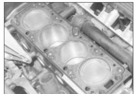
11.22 New head gasket in position
