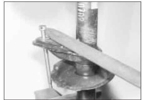
4.6a One method of unscrewing the strut ring nut
