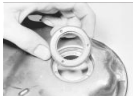
14.14b . . . and refit the holder and seal to the timing cover
