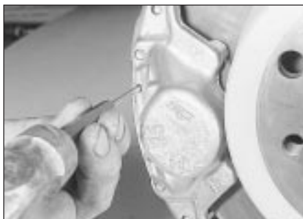
5.3 Driving out a rear disc pad retaining pin
