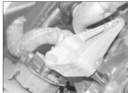
23.20b Engine/transmission right-hand mounting
