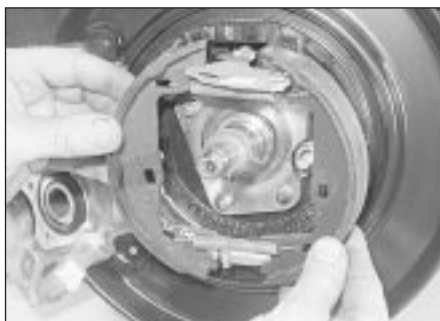
20.4 Removing the handbrake shoe assembly
