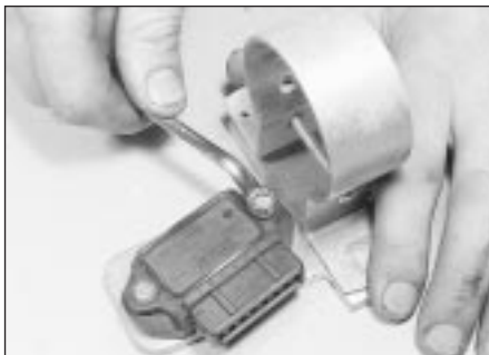
7.3 Unbolting the ignition module (1.8 litre model shown)
