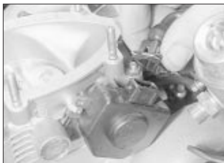
12.82 Disconnecting the throttle valve switch multi-plug
