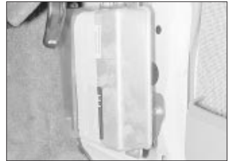
12.48 Motronic control unit location
