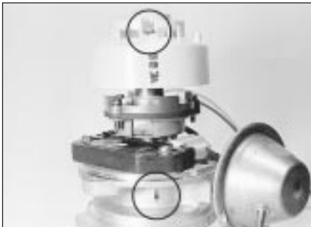
3.19a Distributor rotor contact, and arrow on distributor body (circled) in alignment . . .
