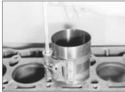
15.12 Piston ring compressor fitted
