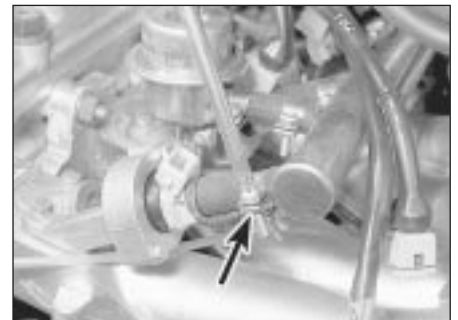
12.6 Slackening a fuel rail hose clamp
