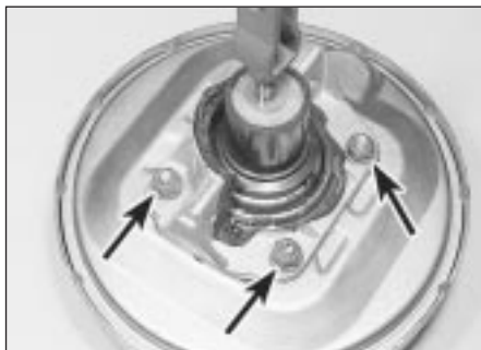
16.9 Three of the four servo-to-bracket nuts (arrowed) servo and bracket removed for clarity
