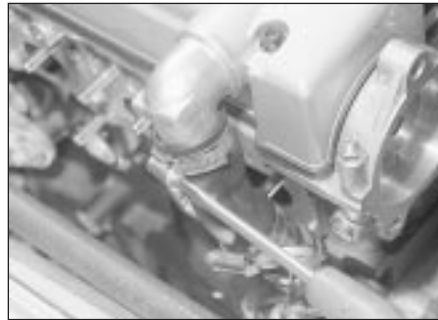
11.15 Disconnecting the large breather hose
