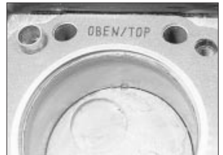
8.22 Head gasket must be fitted with the word OBEN (or TOP) uppermost
