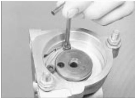
9.5a Removing the Allen screws which secure the camshaft thrust plate
