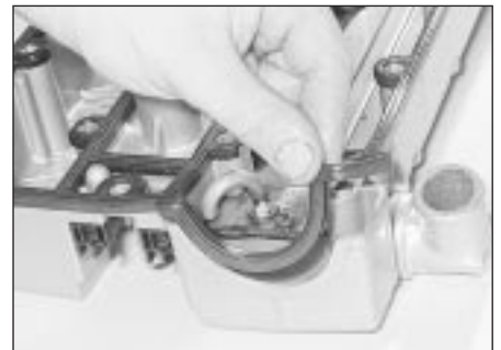
11.25 Fitting a new gasket to the camshaft cover
