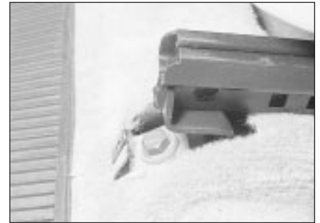
31.2a Seat rail front retaining bolt (one of two)
