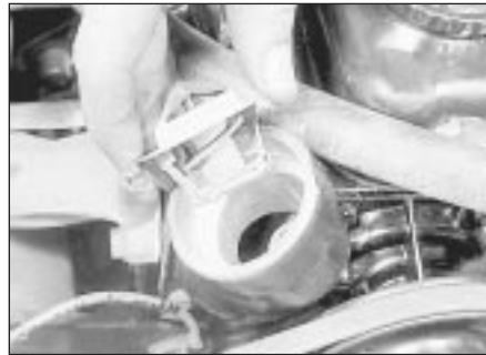
4.3b . . . and withdraw the thermostat - 1.2 litre model
