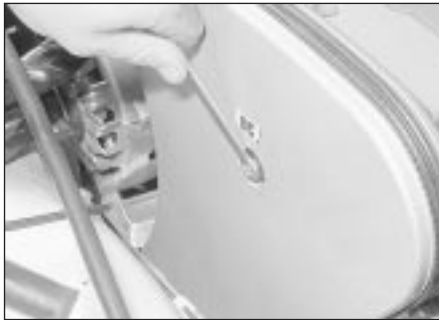
7.6a Removing a belt cover bolt . . .
