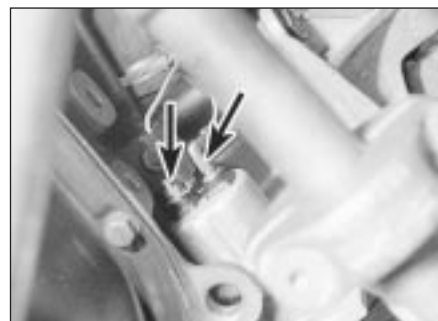
13.2 Oil pressure sender wires (arrowed)
