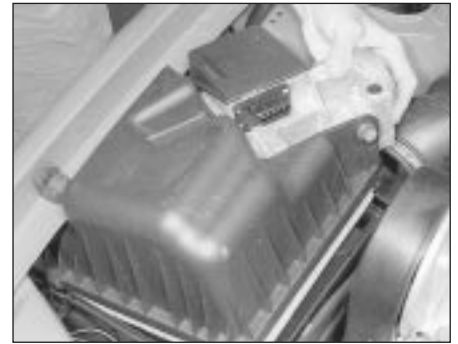
24.8b . . . and remove the air cleaner housing cover, complete with the filter element
