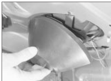
26.2a On Saloon models, unclip the plastic covers to gain access to the underside of the rear speakers . . .
