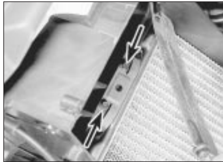
9.17b Heater matrix upper securing screws (arrowed)
