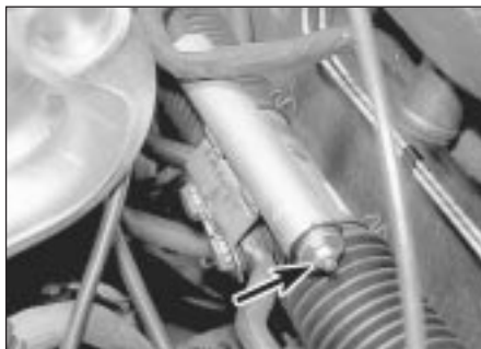
26.2 Steering damper securing nut (arrowed)
