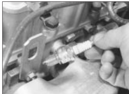
7.5 Removing a spark plug - 1.6 litre engine shown
