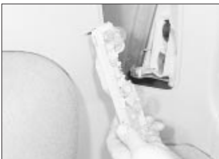
11.16b Rear lamp cluster bulbs and holder
