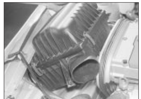
2.5c Removing the air cleaner - 2.0 litre 16-valve
