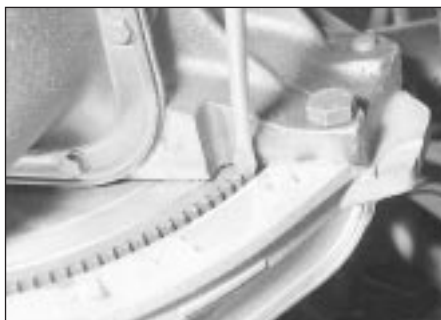
7.4 Jamming the flywheel ring gear
