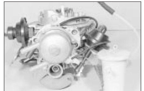
22.2b 2E3 carburettor - choke cover side view
