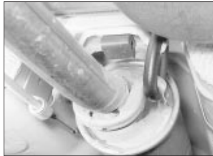
27.4b Exhaust system rubber mounting ring
