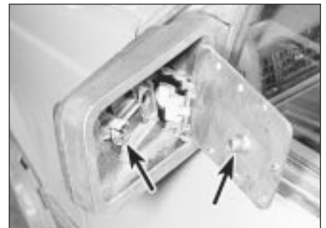
30.2b Engage the linkage and press the ball into the socket (arrowed)
