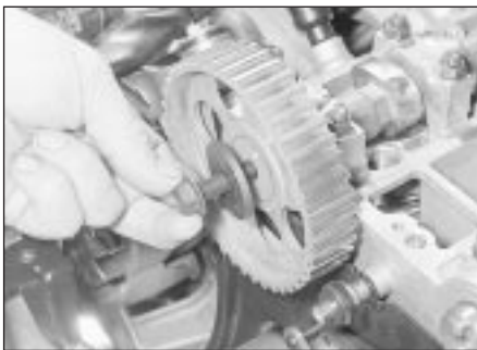
10.3a Removing a camshaft sprocket bolt and washer
