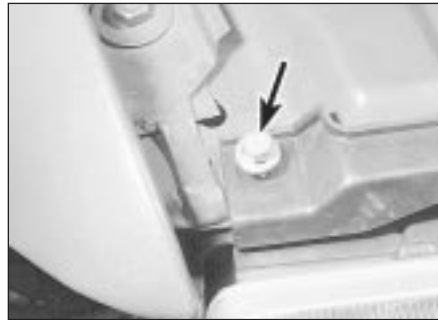
12.3a Headlamp lens outboard securing screw (arrowed)
