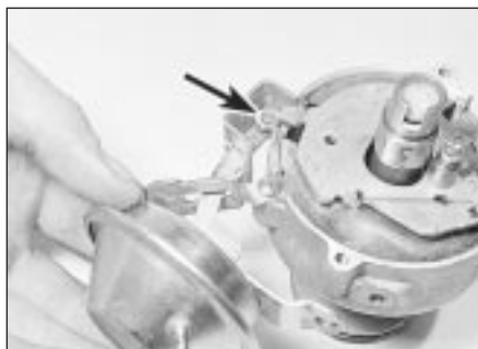
7.6b . . . and disengage the operating arm (arrowed) while withdrawing the unit
