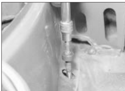
16.8 Removing a servo bracket screw
