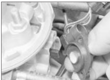
11.3b Throttle valve potentiometer removal
