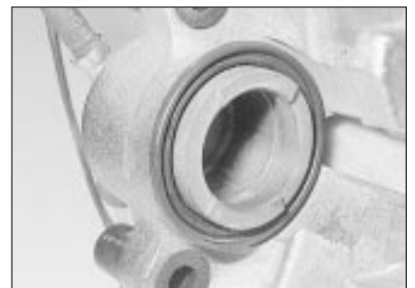
4.23 Prior to fitting the pads, ensure that the caliper steps are positioned as shown
