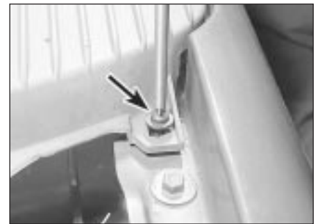
11.3a Wind deflector screw at the wing
