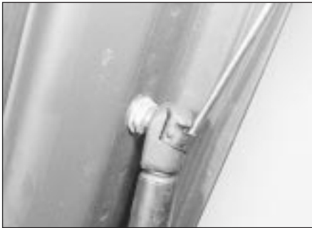
22.2 Releasing a tailgate strut spring clip
