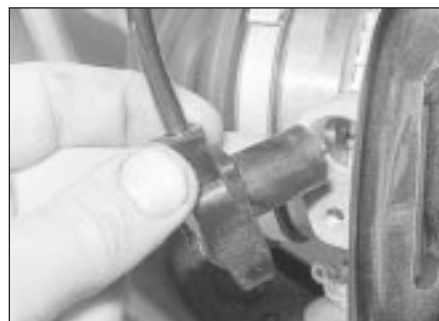
22.2c Removing a front wheel speed sensor
