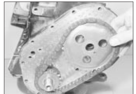
14.11 Removing the sprockets and timing chain
