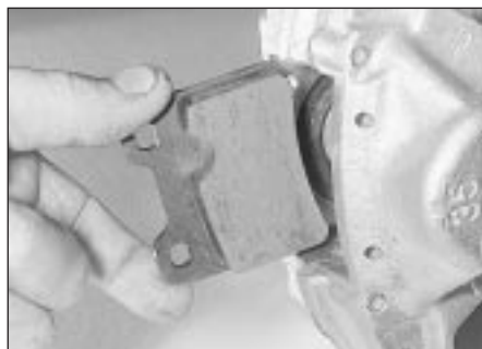
5.9a Fitting a rear pad
