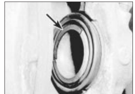
11.8 Correct position of rear caliper piston step, showing the inboard piston step, the opposite piston is the mirror image
