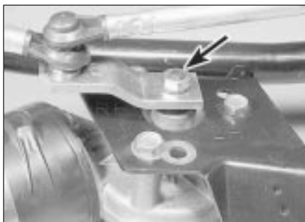
20.8a Wiper motor spindle nut (arrowed)
