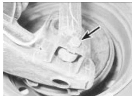
12.5 Rear shock absorber lower mounting bolt (arrowed) - Hatchback
