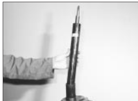
4.7 Removing the shock absorber cartridge
