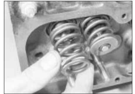
9.18a Fit the valve spring . . .
