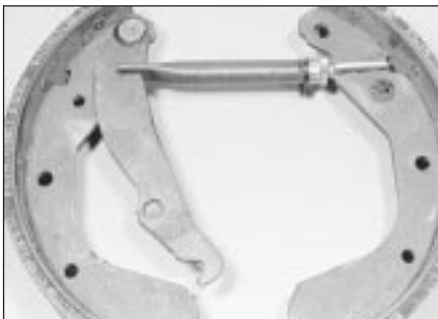
6.17a Self-adjusting strut correctly fitted
