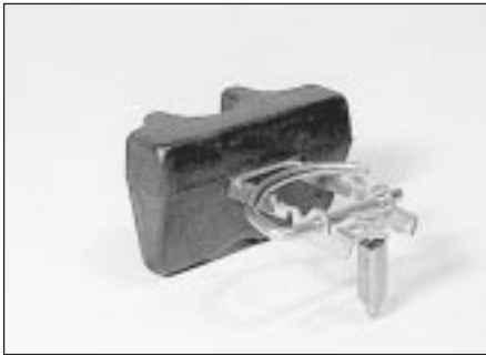
23.13 Float and needle valve
