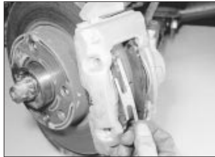
4.4a Removing an anti-rattle spring
