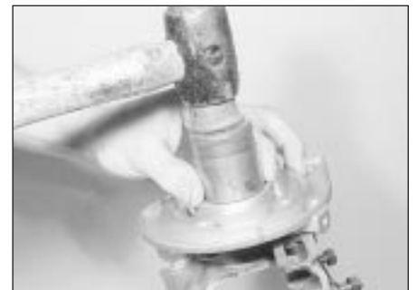
9.8b Fitting a new camshaft housing oil seal
