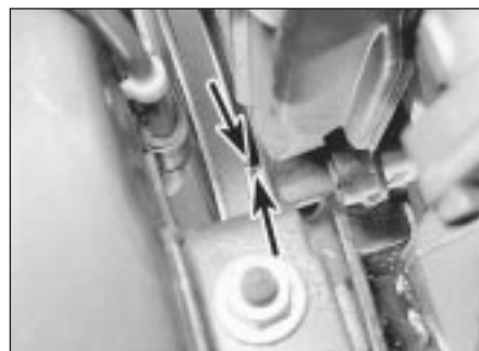
7.2a Crankshaft pulley notch and oil pump pointer in alignment (arrowed)
