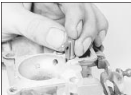
21.8 Removing the accelerator pump delivery tube
