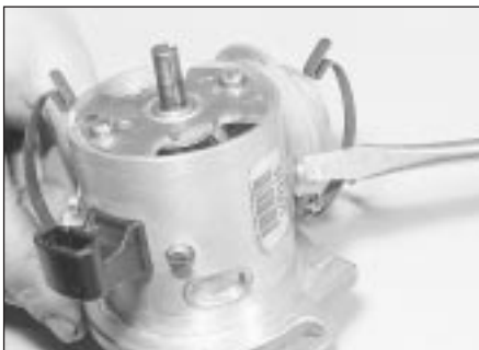
4.16a Removing a vacuum unit retaining screw
