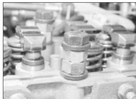
9.3 Cylinder head bolt, with washers and nuts for spacers, used to clamp head
