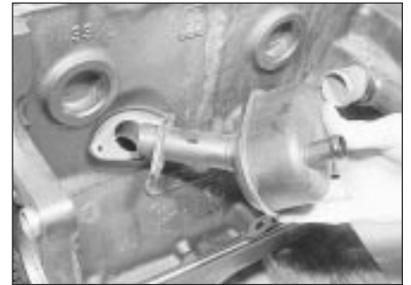
22.8 Crankcase ventilation system oil separator - 1.3 litre engine
