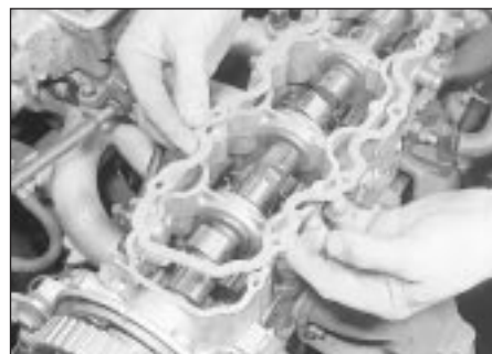
8.29a Fitting a new camshaft cover gasket
