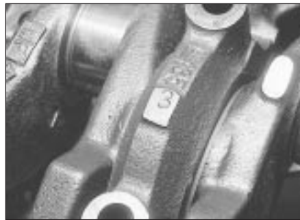
20.3 Identification number on No 3 main bearing cap
