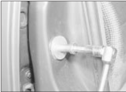
13.4 Adjusting a door lock striker
