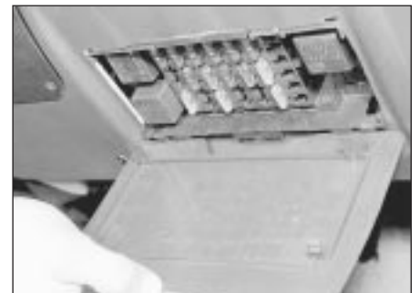
3.1 Removing the cover from the fuse/relay box
