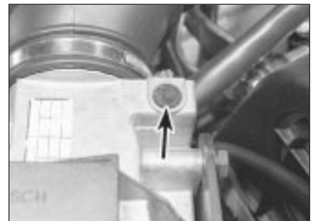
11.13 On 1.8 litre fuel-injected models the mixture adjustment screw is located under the cap on the airflow sensor
