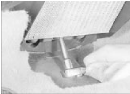
9.17a Removing the heater matrix lower screw
