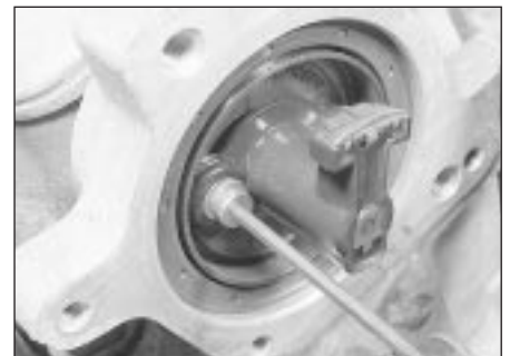
3.10a Undo the two Allen screws . . .
