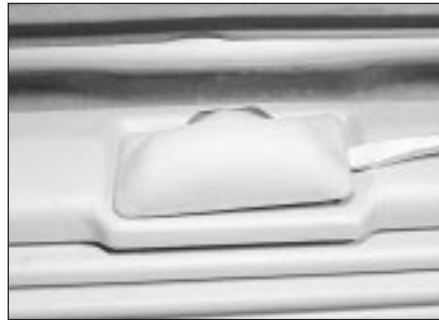
11.22 Prising out the number plate lamp
