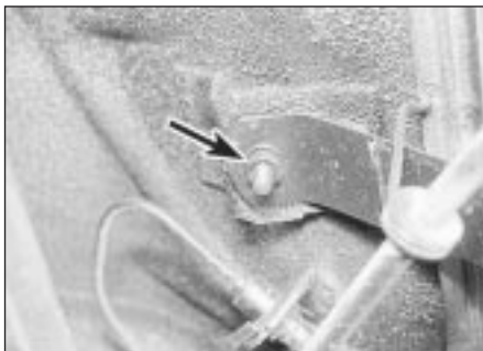
7.12 One of the fuel tank retaining strap nuts (arrowed)
