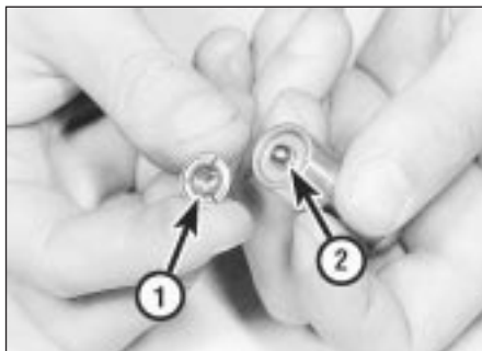
10.13a Spring (1) located in plunger cap, and ball (2) located on seat in plunger
