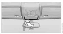
Using the screwdriver, press in the clamps one after the other, arrows 1, tilt the cover panel down, arrow 2, and remove.
