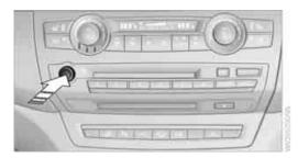
Press the knob if the sound output is switched off.
