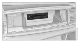
The BMW CD changer for six CDs is installed in the glove compartment.
