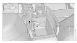
1 Connection for audio playback: TRS connector 1/8 in/3.5 mm
