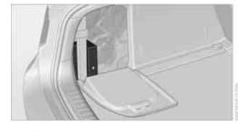
The first-aid kit is located in the cargo bay. Open left side panel, remove warning triangle.
