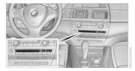
When equipped with two drives: The upper drive is for audio CDs.
