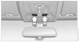
Reading lamps are provided in the front and rear\* adjacent to the interior lamps. Press the button to switch the lamps on and off.
