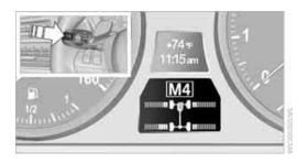
Press the BC button on the turn signal lever repeatedly until the display appears, refer to arrow.
