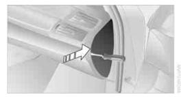
Pull the strap upward, arrow. The glove compartment is opened manually.
