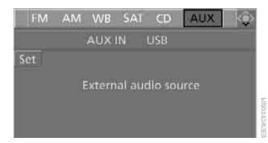
Select "USB" or the name of the audio device and press the controller.
