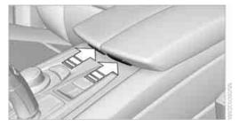
Push cover down slightly and press the button. The cover folds upward.
