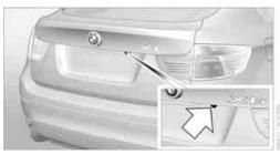
The lens of the rear view camera is located on the liftgate.
