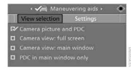
Select "PDC in main window only" and press the controller.
