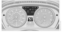
The indicator and warning lamps can light up in different combinations and colors.
