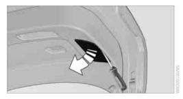
Rotate the bulb socket to the left and remove.
