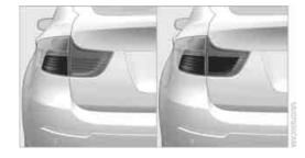
On the left: normal braking. On the right: heavy braking.
