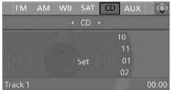
Change to the second field from the top if necessary. On vehicles with a CD changer, select "CD" and press the controller to start the CD player.
