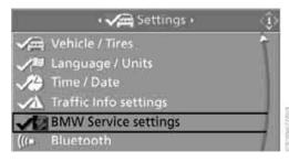
Change to upper field if necessary. Turn the controller until "Enabled services" is selected and press the controller.
