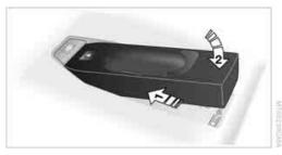
To remove the snap-in adapter: Press down on region **1**.
