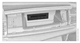
The BMW DVD changer for six DVDs is installed in the glove compartment.
