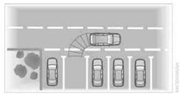
Turn the steering wheel so that the pathway lines cover the corresponding turning lines.
