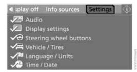
Select "Vehicle / Tires" and press the controller. Change to upper field if necessary. Turn the controller until "TPM" is selected and press the controller.
