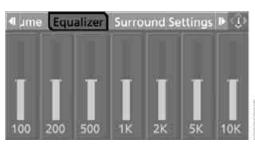
2. Move the controller to the left or right to select the desired frequency range.
