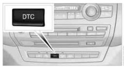
Press the button until the DSC indicator lamp in the instrument panel lights up, but not longer than approx. 10 seconds. DTC Dynamic Traction Control and DSC are deactivated together. Stabilizing interventions are now not carried out.
