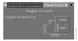
6. Change to the second field from the top if necessary. Turn the controller until "Engine oil level" is selected and press the controller. The oil level is displayed.
