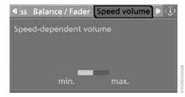
Turn the controller: The adjustment is applied; the field can be changed.
