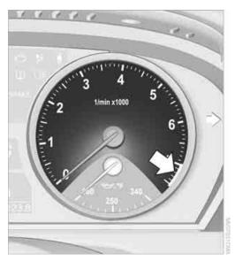
Do not operate the engine with the needle in the red overspeed zone of the gauge, refer to arrow. At high revs in this range, the flow of fuel is interrupted to protect the engine.
