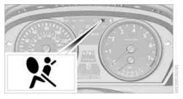
From radio readiness, refer to page 56, the warning lamp lights up briefly, indicating the operational readiness of the entire airbag system and the safety belt tensioners.
