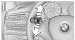
Press the button in the turn signal lever up or down.
