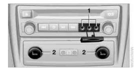
Connections for audio/video cables: Watch the colors of the sockets when connecting.
