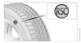
You will recognize run-flat tires by the circular symbol containing the letters RSC on the side of the tire.
