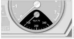
When the engine is at operating temperature, the engine oil temperature is between approx. 170 °F/80 °C and approx. 250 °F/120 °C.
