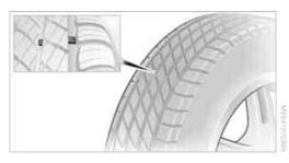
Wear indicators at the tread-groove base are distributed over the tire's circumference and are marked on the side of the tire with TWI -Tread Wear Indicator, If the tire tread has been driven down to the wear indicators, a tread depth of 0.063 in/1.6 mm has been reached.
