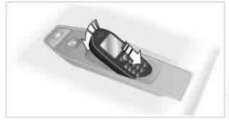
The mobile phone battery is charged from the radio readiness position.
