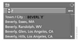
Change to the third field from the top if necessary. Turn the controller until the town/ city name is selected from the list and press the controller.
