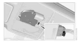
4. Take the Allen wrench\* from its bracket in the onboard tool kit, refer to page 245, and insert it into the opening provided. Move the glass sunroof in the desired direction.
