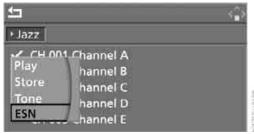
Select "ESN" and press the controller. The electronic serial number, ESN, is displayed.
