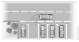
The pathway lines are dependent on the current steering angle and are continuously adjusted to the steering wheel movements.
