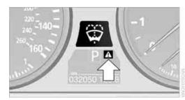
▲ means that a Check Control message has been generated. The symbol continues to be visible even when the Check Control message disappears after a short time. The warning lamps and text messages are stored and can be displayed later, also refer to page 76.
