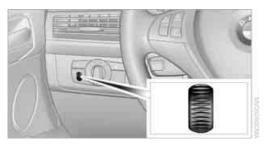
You can control the lighting intensity by using the knurled wheel.
