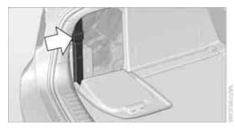
The warning triangle is located in the cargo bay. Open the left-hand side panel.
