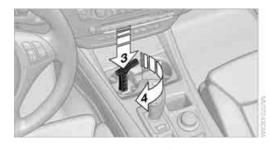
Turn the releasing tool as far as possible, arrow 4, and then press downward and leave it in. The transmission lock is released.
