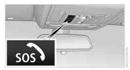
Press the button for at least 2 seconds.The BMW Assist Response Center is contacted.
