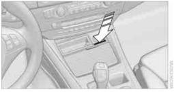
Press the button. The ashtray insert raises slightly and can be removed.
